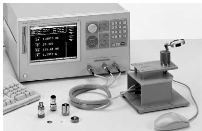
Agilent 4287A RF LCR meter 1 MHz to 3 GHz
