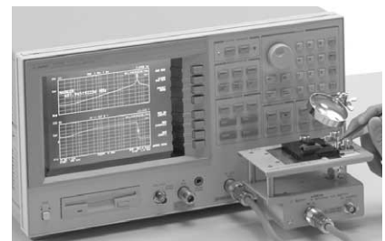
Agilent 4396B network/spectrum/impedance analyzer 100 kHz to 1.8 GHz/2 Hz to 1.8 GHz/ 100 kHz to 1.8 GHz
